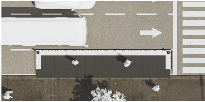
PLATFORM AS AN EXTENSION OF THE SIDEWALK.
