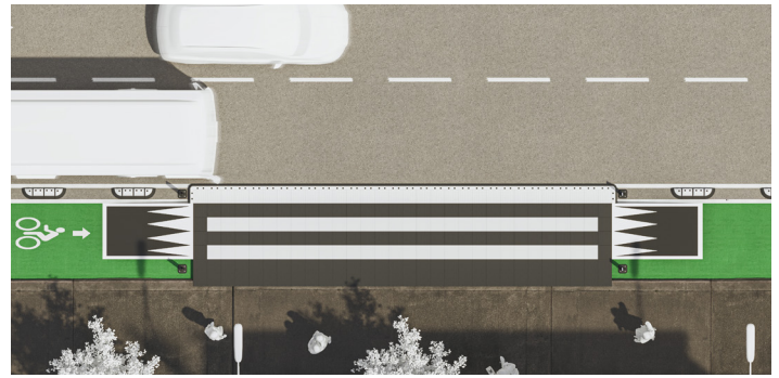
PLATFORM WITH INTEGRATED CYCLE LANE.
