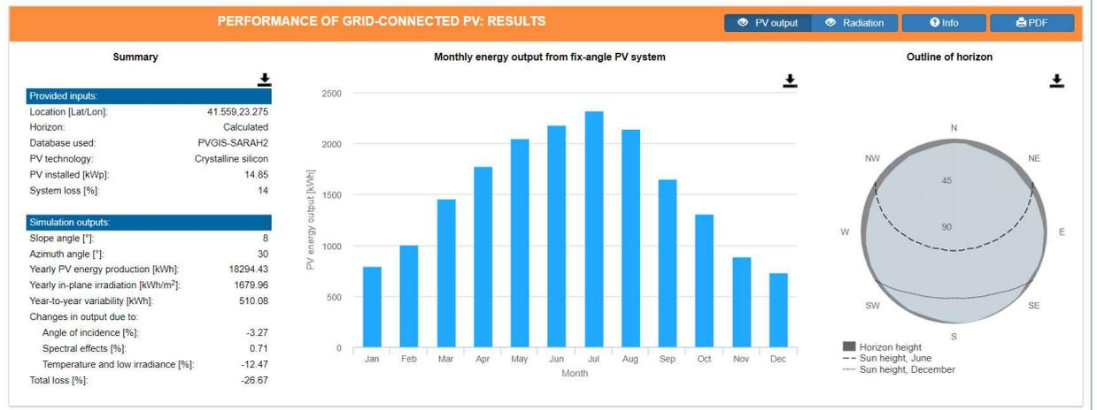
**Fig. 5.1.** An overview of the results for a sample photovoltaic system
