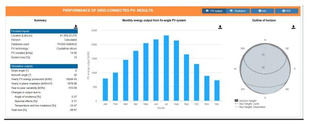
Fig. 5.1. An overview of the results for a sample photovoltaic system
