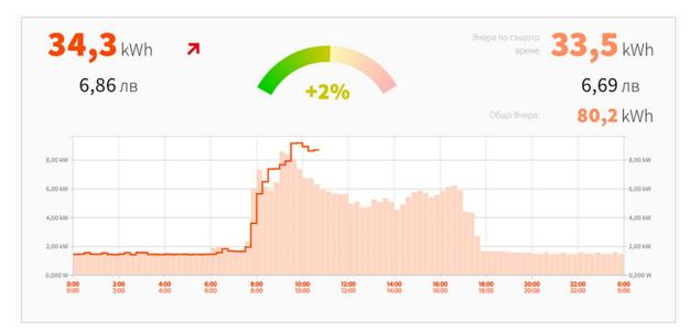
Fig. 3.2. Sample daily load profile of one electricity circuit of an office building
